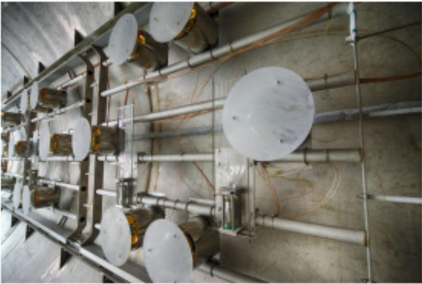
Figure 29. Left: diagram of the optical unit; Right: units mounted in MicroBooNE, immediately prior to LArTPC installation.
