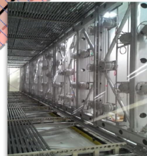
360 PMTs behind the wires to collect scintillation light and trigger events
