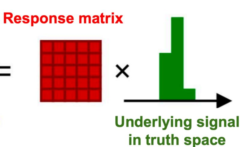
We use a regularization technique to avoid large fluctuations after inversion
