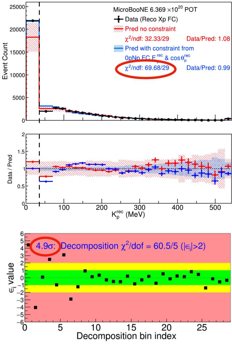
This decomposition test transforms the covariance matrix and  $\chi^2$  calculation to a space where the bins are uncorrelated
